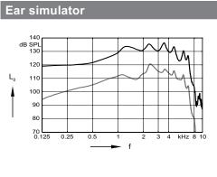
Output sound pressure level (L<sub>i</sub> = 90 dB)
