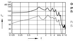
Output sound pressure level (L<sub>i</sub> = 90 dB)
